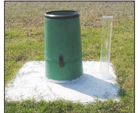
Rain Gauge (non-recording) Use: Measurement of Rainfall (mm)
