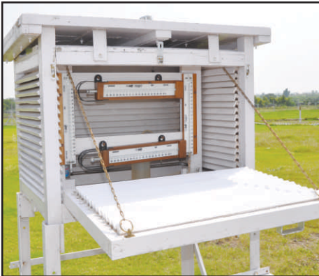
Thermometers (Maximum, Minimum, Dry Bulb & Wet Bulb) inside Single Stevenson Screen Use: Recording of Maximum and Minimum Temperature ( ^{\circ}\text{C} ), Rel. Humidity (%)
