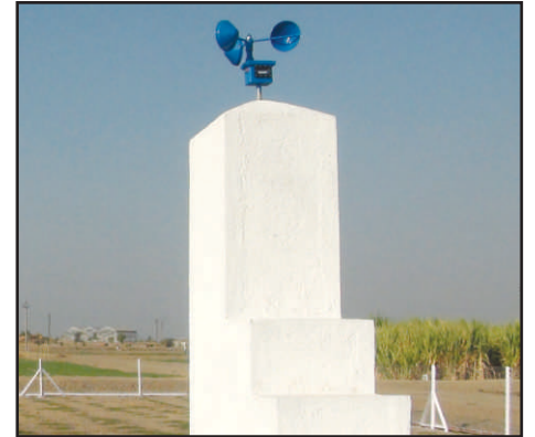
Cup Counter Anemometer Use: Measurement of Wind Speed ( \text{Km hr}^{-1} )
