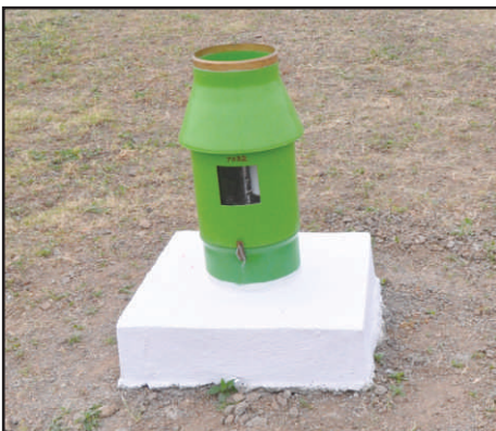
Rain Gauge (self-recording) Use: Measurement of Rainfall (mm)
