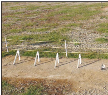
Soil Thermometers Use: Recording of Soil Temperature ( ^{\circ}\text{C} )
