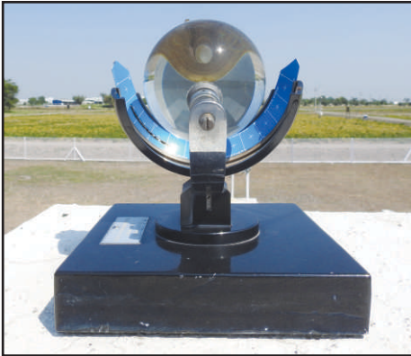
Campbell Stokes Sunshine Recorder Use: Recording of Bright Sunshine Duration (hrs)
