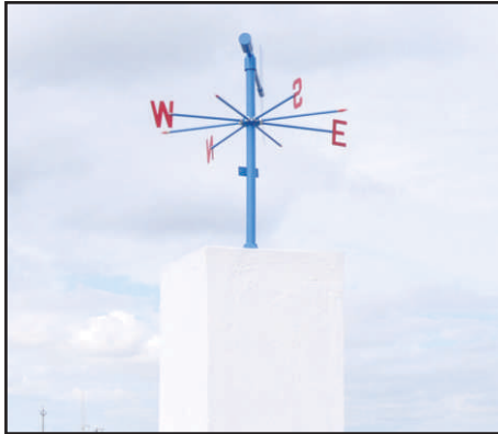
Wind Vane Use: Indication of Wind Direction
