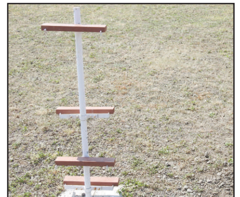
Dew Gauge Use: Measurement of Dew amount (mm)
