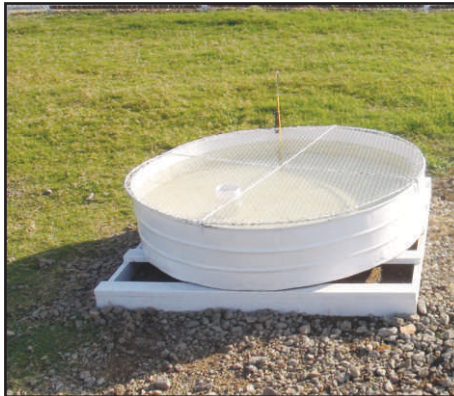
Pan Evaporimeter Use: Measurement of Evaporation (mm)
