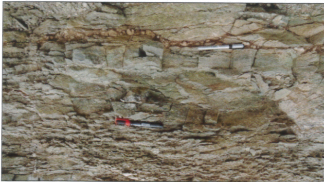
Fig.30. Amygdular (vesicular) and normal (nonvesicular) flows are separated with thin beds of scoriae or inter-trappean beds, upper portion (vesicular flows) of the trap is showing weathering effects
