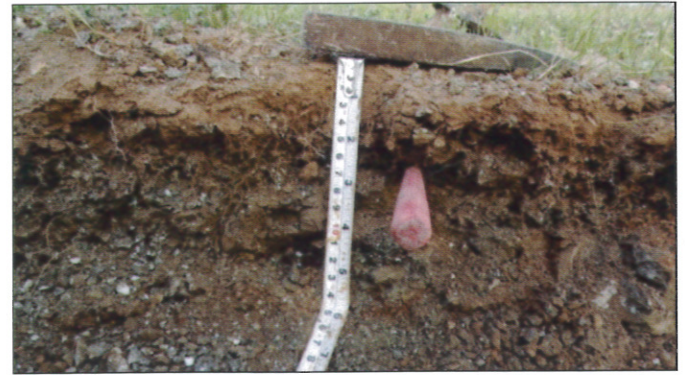
Fig.53. Profile developed on backslope, 12 cm deep, A horizon 4-6 cm underlain by R horizon with gravelly loamy sand texture (Profile 4)
