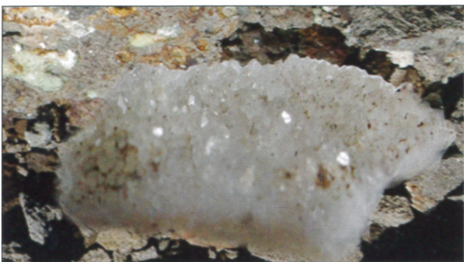
Fig.35. Sample showing the growth of sheaf-like aggregates of well developed zeolite crystals
