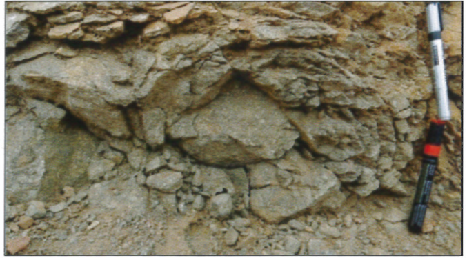
Fig.43 Enlarge view of the spheroidal weathering showing the hard unaltered core of trap rocks
