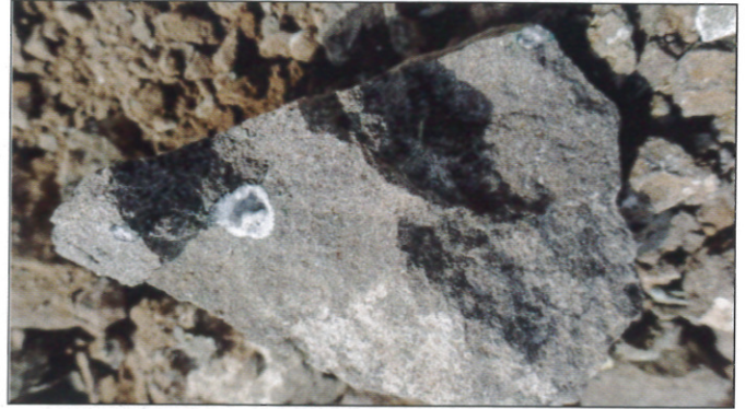
Fig.31. Sample from upper part of normal (nonvesicular) flow, dark gray in colour, consisting of fine grained basalt filled up with secondary precipitates of silica
