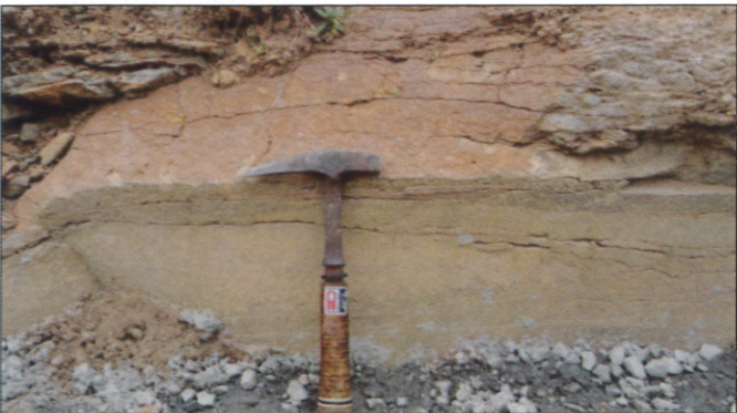
Fig.24. Upper part of normal (nonvesicular) flow consisting of fine grained weathered basalt
