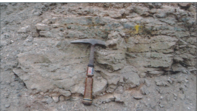
Fig.25. Upper part of normal (nonvesicular) flow consisting of fine grained weathered basalt
