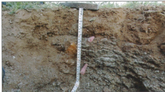
Fig.52. Profile developed on shoulder slope, 23 cm deep, A horizon 8-10 cm underlain by C horizon of 12 cm (10-22cm) and followed by R horizon with gravelly sandy loam in texture (Profile 3)
