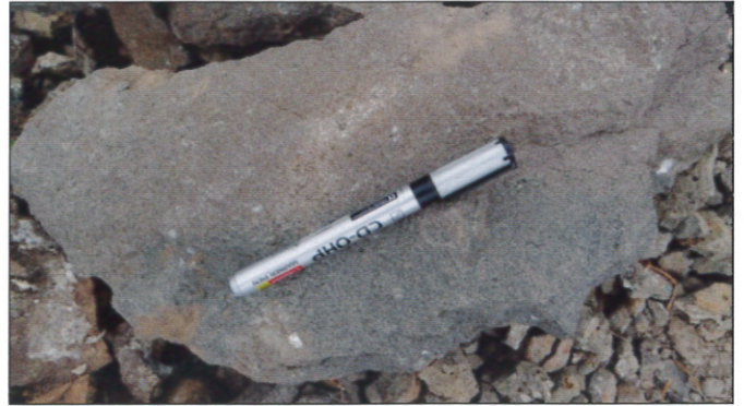
Fig. 26. Upper part of normal (nonvesicular) flow consisting of fine grained basalt, colour gradation is due to differential leaching or magmatic fractionation
