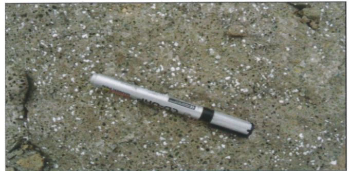
Fig.12. Sample from lower part of amygdular flows, cavities are very small and many and filled up with zeolite minerals indicating that lava was cooled down very quickly with lots of gaseous emanations which also indicates the hydrothermal activities were highly active
