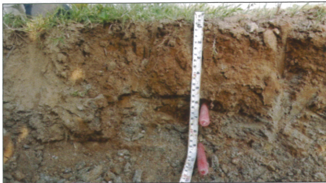
Fig.51. Profile developed on side slope, 24 cm deep, A horizon 14-15 cm underlain by AC horizon of (15-23 cm) 8 cm and followed by C horizon, with sandy clay loam texture (Profile 2)
