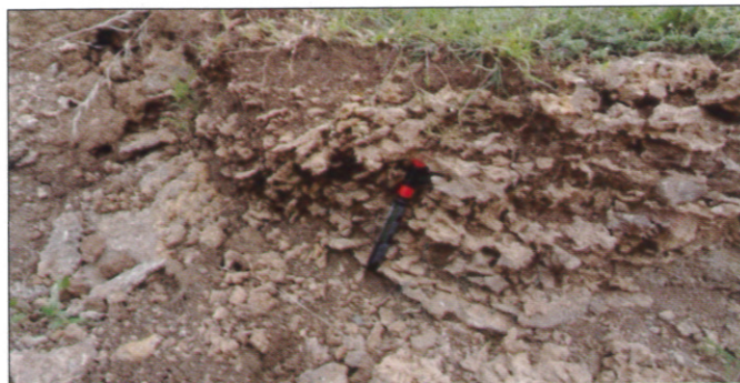
Fig.47. Formation of skeletal box work structure during the weathering of profile, soft portion has been removed and harder portion forming the skeletal like structure, the profile is intercalated with soil matrix
