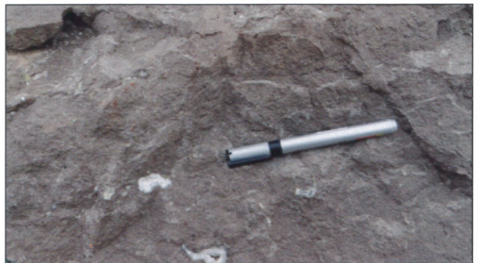
Fig.27. Sample from upper part of normal (nonvesicular) flow consisting of fine grained basalt, cracks filled up with secondary precipitates of silica
