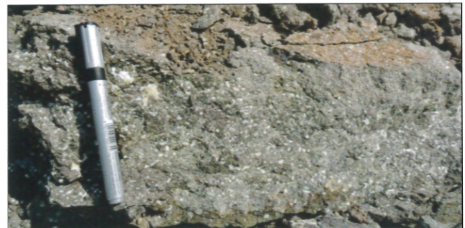
Fig. 13. Sample from lower part of amygdular flows, cavities are filled up with zeolite minerals, brownish colour of the sample indicates the effects of leaching
