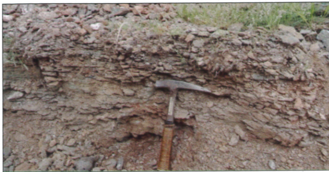
Fig.46. Weathering of rocks along the fractures and cracks from upper to lower horizon of vesicular flow
