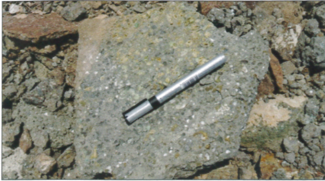
Fig. 15. Sample from lower part of amygdular flows, cavities are filled up with different types of zeolite minerals
