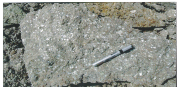
Fig.14. Sample from lower part of amygdular flows with increase in ferromagnesian minerals it is tending towards the formation of laterite, cavities are filled up with different types of zeolite minerals
