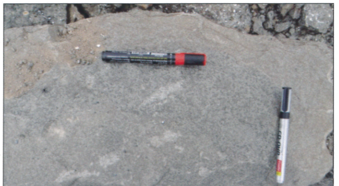
Fig.28. Sample from upper part of normal (nonvesicular) flow consisting of fine grained basalt, the brown colour of the rind and light brown colour at the periphery is due to differential leaching
