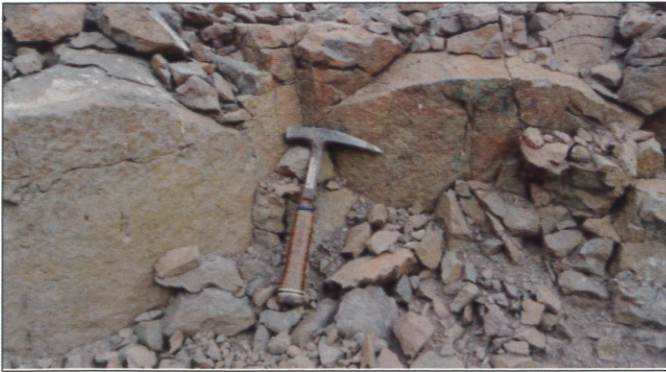
Fig.22. Upper part of normal (nonvesicular) flow consisting of fine grained, hard and compact basalt
