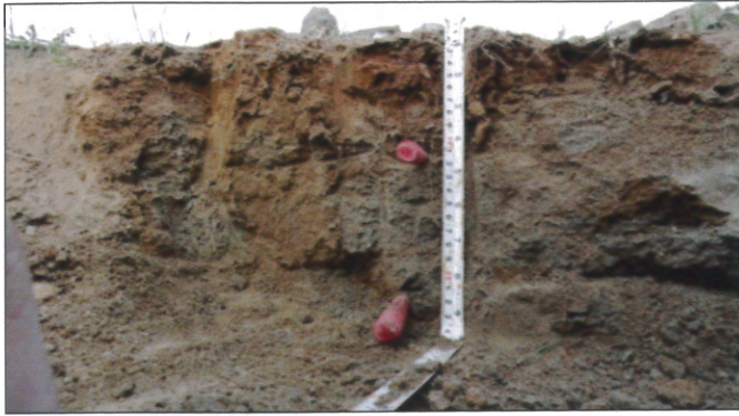
Fig.50. Profile developed on summit. 24 cm deep, A horizon 10-12cm underlain by AC horizon of 11 cm and followed by C horizon with sandy loam texture (Profile 1)
