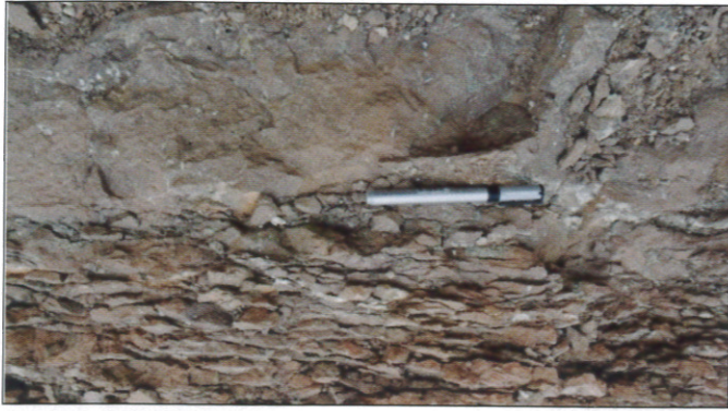
Fig 29. Middle part of vesicular and upper part of nonvesicular flow occurs together, vesicular flows are hard and massive while nonvesicular flow showing the weathering effect
