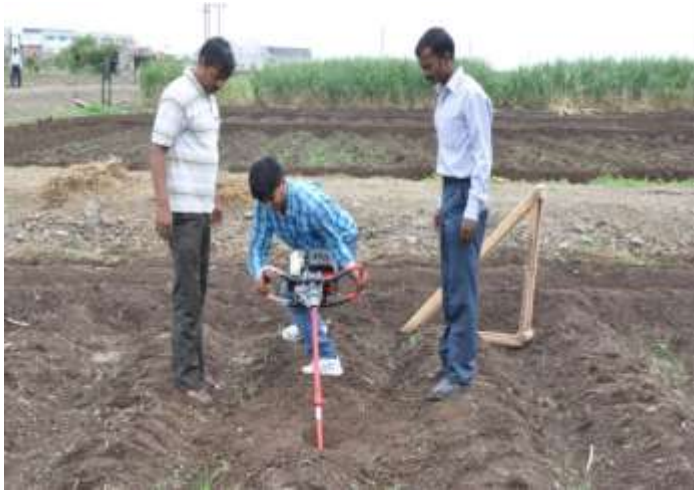
Fig. 3. Motorized root auger for digging the hole in the soil, and transparent acrylic tubes are inserted into the holes
