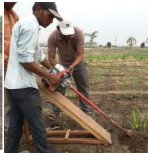
Fig. 4. Wooden platform for guiding the motorized root auger.
