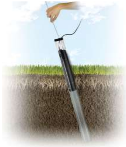
Fig. 1. CI-600 scanner for in-situ root image recording.
