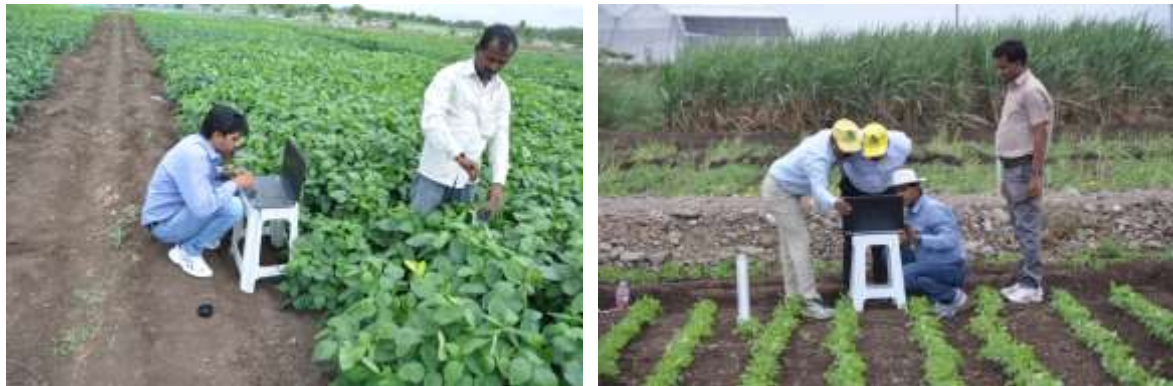
Fig. 5. In-situ root image acquisition by using CI-600 root scanner.
