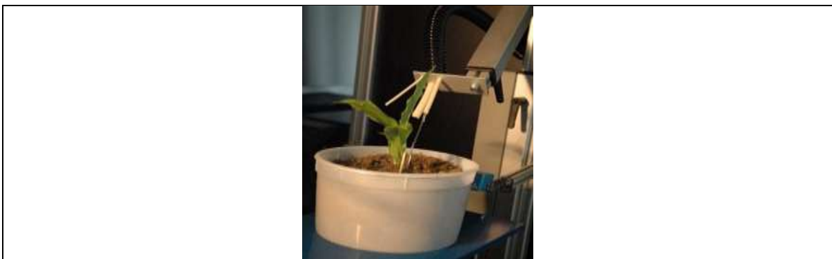
Fig. 1. Watering and watering station. Plants are lifted pneumatically from the belt to obtain precise weights.
