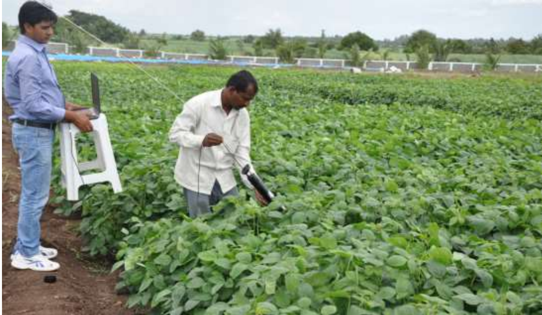
Fig. 1. CI-600 scanner for in-situ root image recording.
