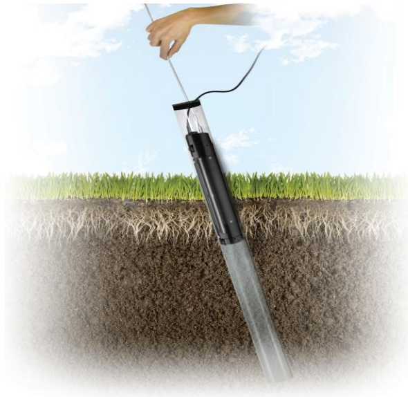
Fig. 1. Mini-Rhizotron for in-situ root image acquisition
