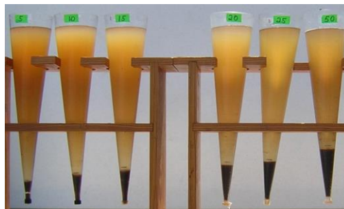
Fig: Imhoff cones, 25-50 ml/l solid requirement for Tilapia biofloc system
