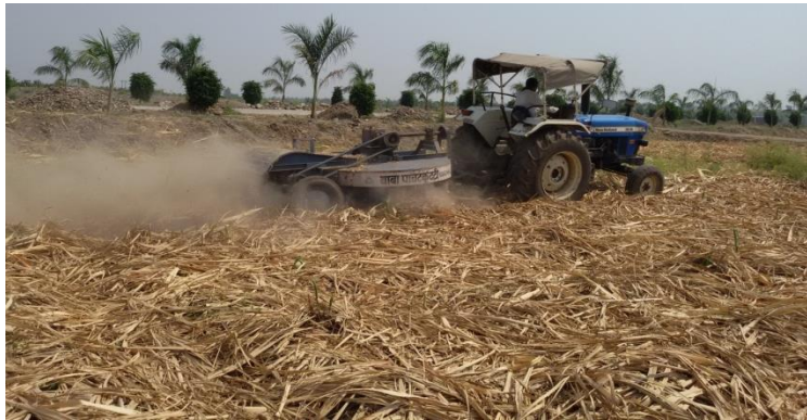
Fig. 2. Photograph showing working of trash cutter
