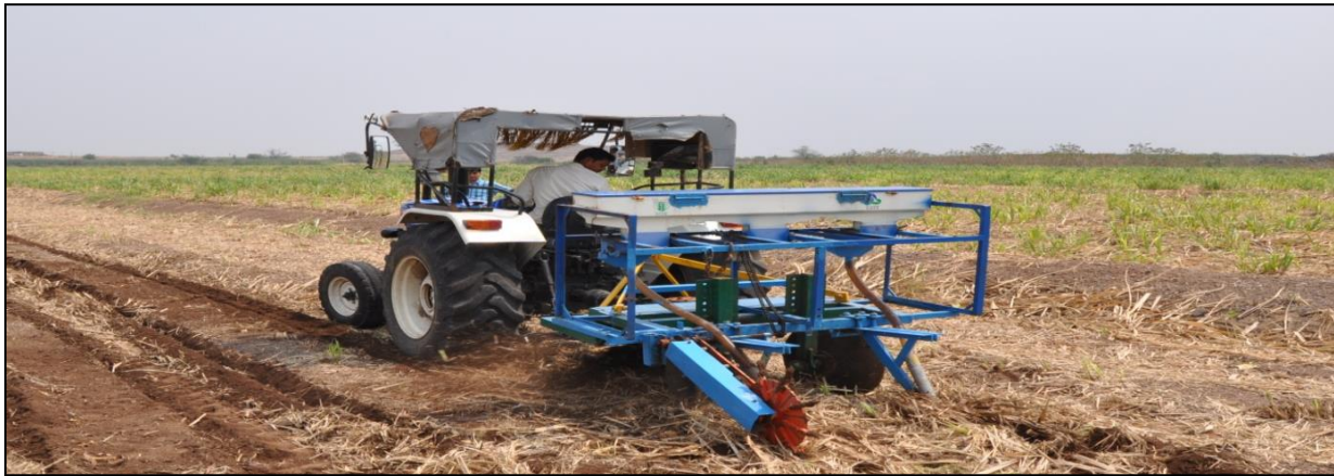
Fig. 3. Photograph showing working of multi-purpose SORF machine
