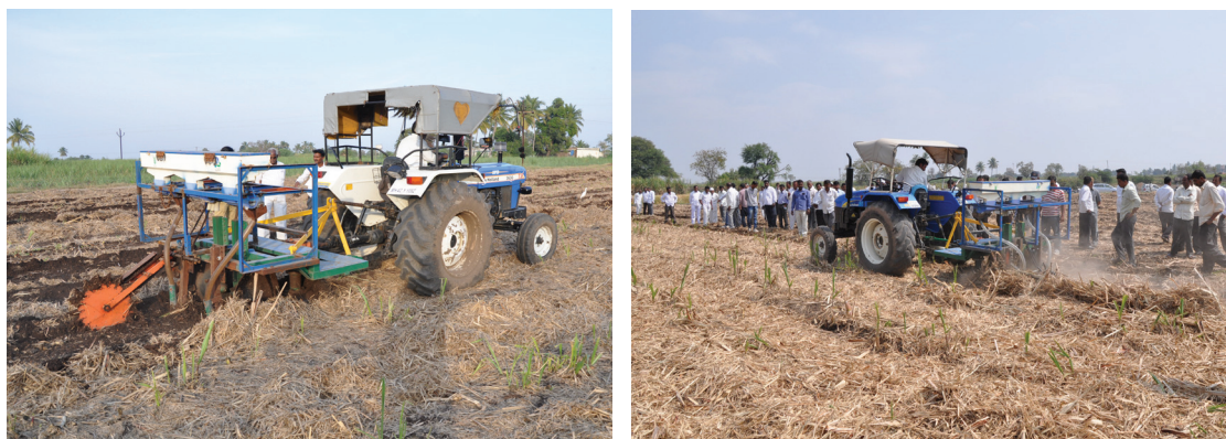
Fig. 2.27. Demonstration of stubble shaver, off-bar, root pruner cum fertiliser drill (SORF) machine at farmers' field
